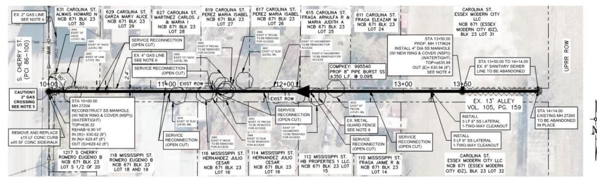
• Upstream dead-end manhole of Compkey 995540 is located under a large shed. This manhole will be abandoned and a new manhole will be installed as shown in the plans.
